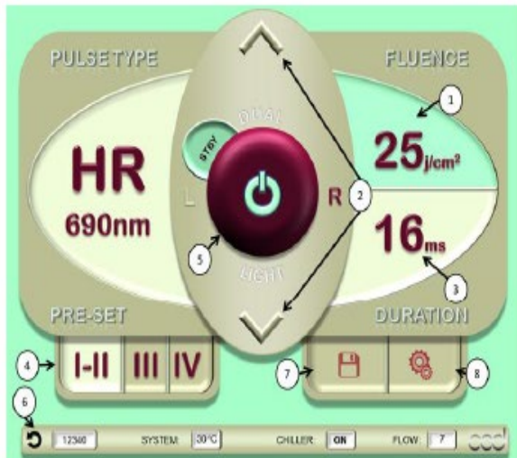
SR/HR Standby Screen
